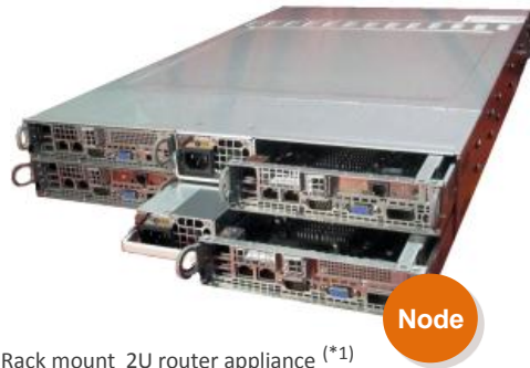
Rack mount 2U router appliance (*1) with 4 router nodes installed
